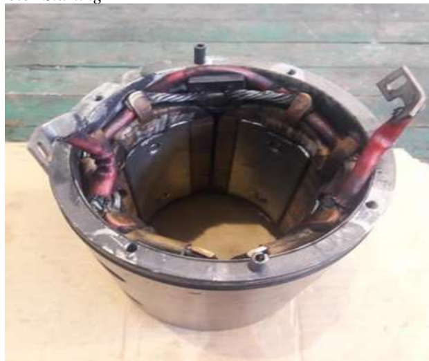
Gambar 8. Hasil Visual Inspection kondisi field welding
