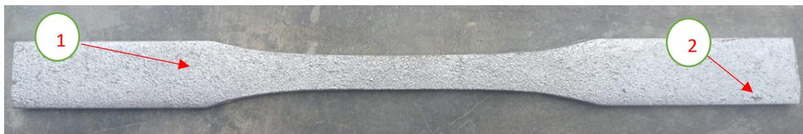
**Gambar 9.** Spesimen 3 Pasir Pantai, Aluminium, Kaleng Bekas
