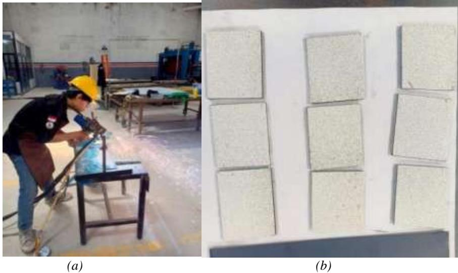
**Gambar 3.** Proses (a) *thermal spray aluminium* dan (b) hasil *thermal spray aluminium*
