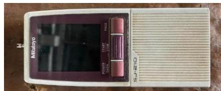
**Gambar 6.** *Surface roughness tester*
