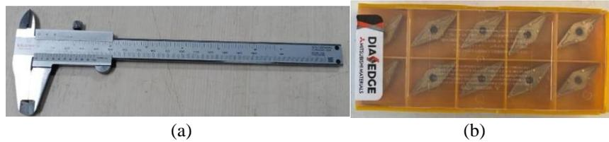
**Gambar 4.** Peralatan (a) Jangka Sorong; (b) Pahat *Insert*
