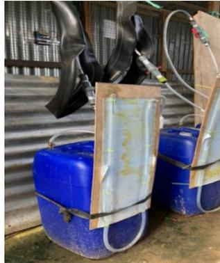
**Gambar 2.** Prototipe digester
